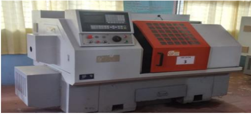
Gambar 7. Mesin CNC Turning NX-L300
